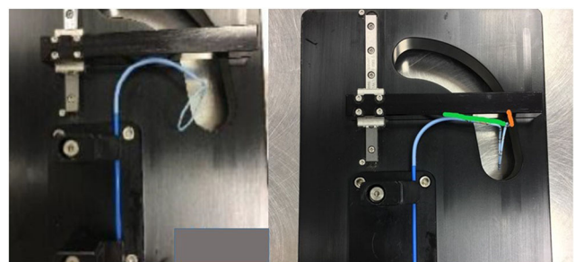
Fig. 4 Original equipment manufacturer (OEM) tests against a template. The “ D curve” of the circular mapping catheter is tested; the annotated green line measures the angle created by the shaft of the catheter. The orange line represents the angle of deflection from the catheter tip and has to be greater than 0 to pass the test
